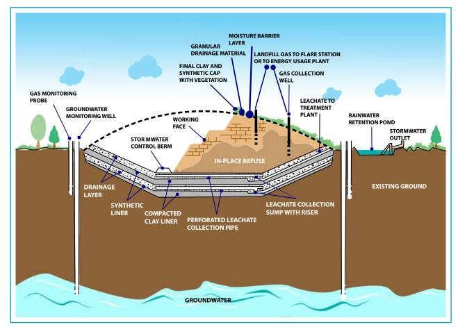
Figure 8: Schematic diagram of a landfill site
